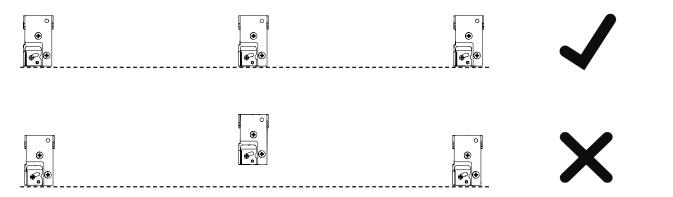
STEP 3 - ATTACH DRAPE TRACK (ASSEMBLED) TO CEILING BRACKETS
