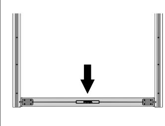
2 Align weight bar with bottom limit and secure latch to U-Mounting Rail on both sides
